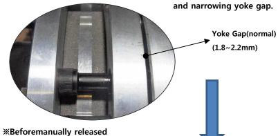
**\*\*Beforemanually released Bolt head is attached to Friction Disc (back panel)**
