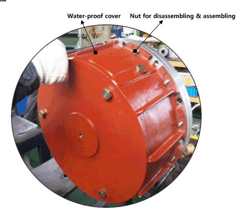
1-1. Disassembling water-proof cover - Separate the cover from the body by disassembling all the nuts as shown above.
